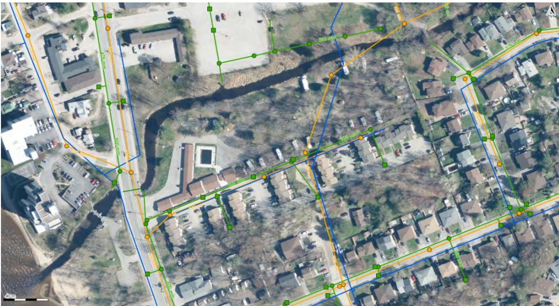
Figure 2 - Parks Creek municipal linear infrastructure (outlet at Lake Nipissing). Blue line signifies watermain; green line signifies storm sewer; orange line signifies sanitary sewer.
