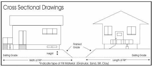
Cross sections must show existing and final grade elevations, existing and proposed finished floor elevations, and lowest openings into buildings.
